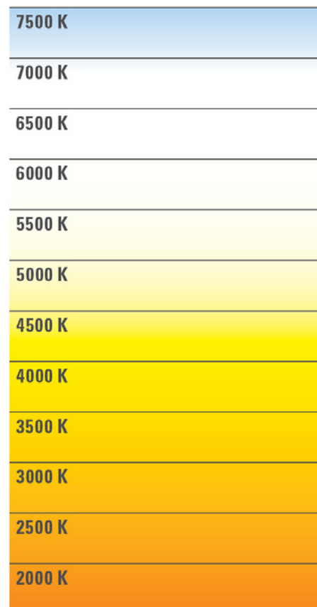
Figure 5. Visual depiction of CCT values shows low CCT values are considered “warm” and high CCT values are considered “cool.”
